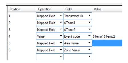
Here, we are mapping the two parts of the Event Code into a temporary variable. Then using the value, we assign them to the Event Code. By placing them straight after each other in the value field, they are concatenated together. So, "F" and "A" becomes "FA".
