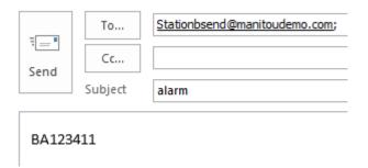
Only the body of the above email contains alarm data. The string in the email body contains the following text without punctuation Separators or spaces:
