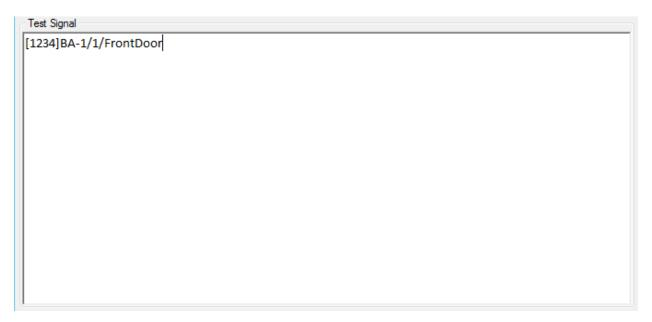
We want to use pre-processing to transform punctuation items acting as Separators into hyphens. The only exception to our mission relates to the first "[" bracket character in the signal. Because that character does not perform a Separator function and needs to be deleted, it requires a greater understanding of Regular Expressions than do the other pre-processing actions we have already performed.
