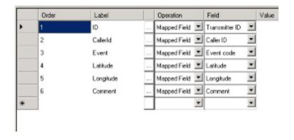
**Note:** there are eight pieces of alarm data in the signal, and only six of those fields have been mapped. We omitted the "Line" and the "GPS EvType" fields from our Data Map because it is not necessary for Manitou to receive that information. It is possible to simply leave the fields out of the Data Map because the XML/JSON Mapping Type only looks for items with the labels you designate in the Data Map.
