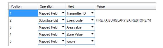
To achieve this, we create a Substitute List as shown above. Use a comma to separate the items, and a colon to link the substitutions.
