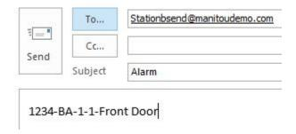
There is no alarm data in the subject of this email, and there is no attachment. All the usable alarm data is contained in the email body only. Each piece of data is separated by a hyphen. Data Mapping is still necessary, however, because Manitou does not know the fields to which each data piece belongs.
