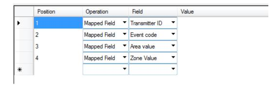
Fields in the "Position" column are numeric, and specify the order in which the fields should be processed.
