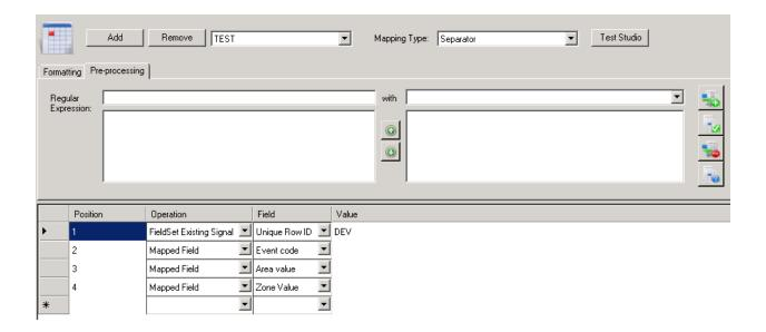
Use the Pre-processing Tab to define alternative forms in which a signal could arrive. For example, if you designated a comma as the Separator for a signal on the Formatting Tab, but you know that the signal might also arrive using a semi-colon, you can prepare Manitou for the arrival of the alternate signal by using the Pre-processing Tab.
